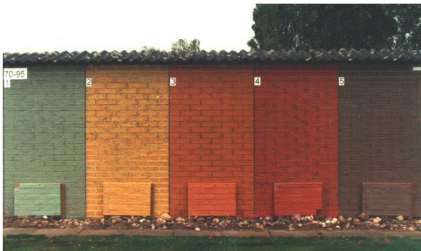
Photo 6: Calcium silicate bricks (un-weathered reference samples in foreground) Weathering commenced: 1970, Photo taken: 1995
