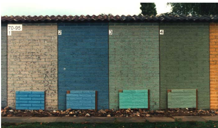
Photo 11: Calcium silicate bricks (unweathered reference samples in foreground) Weathering commenced: 1970, Photo taken: 1995)
